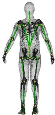
Original undeformed mesh displayed with rigid and soft tissues. Green lines denote segments, yellow dots denote joint center locations about which rotations are defined.
